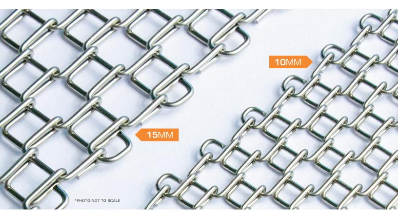
Compact-Grid<sup>™</sup> is designed to offer superior support for small products. Compact-Grid's 70% open surface area makes it easy-to-clean and offers exceptional flow-through properties for heating, cooling, and coating operations. Compact-Grid's no-slip positive drive provides the highest standard in belt tracking, which means the belt will run straight and true even under heavy loads.
