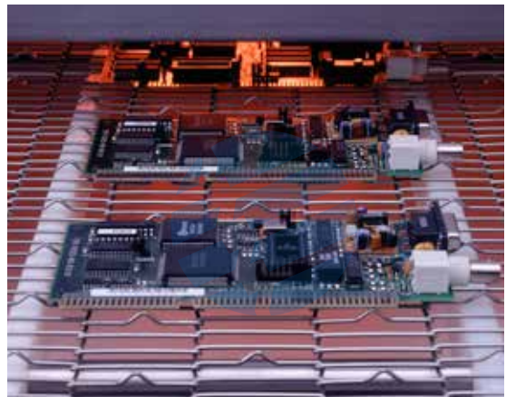
Printed circuit board handling for minimum contact point support
