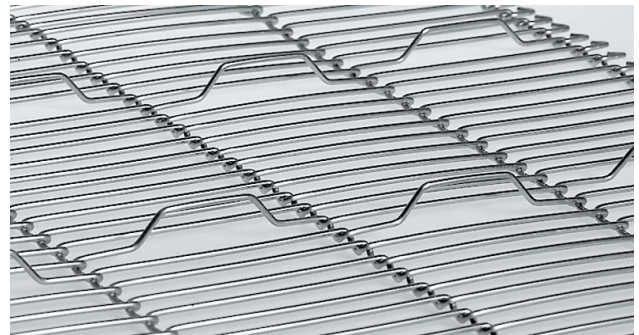
Aligned belts utilize rows of flights (highlighted) to permit control and separation of delicate products
