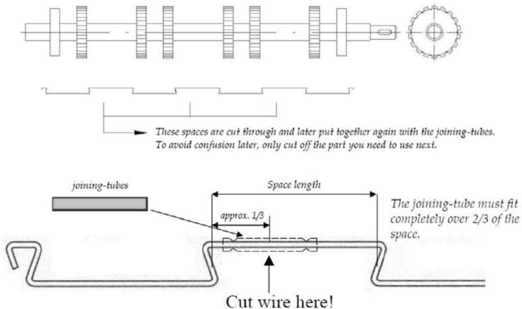
JOINING TUBES are available from Wire Belt Company to suit all belt wire diameters. Please contact our Customer Service Team.
