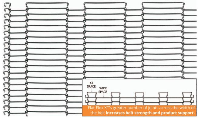
When you require EXTRA strength and support from your conveyor belt look no further than **FLAT-FLEX® XT®**. XT's unique smaller spaces increase the amount of joints across the width of the belt making the belt stronger. XT's unique design enables superior distribution of product weight across the width of the belt, reducing metal fatigue and increasing belt life.
