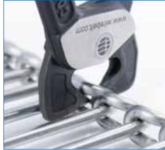
Insert the belt maintenance tool's jaws into the belt edge.
