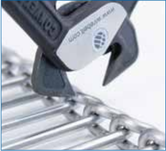
Insert the belt maintenance tool's jaws into the belt edge.
