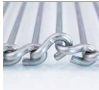
Connect the belt edge by hooking the edge over the strand.
