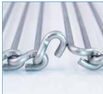
Connect the belt edge by hooking the edge over the strand.
