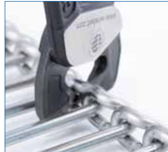
Close down the handle to open the belt edge.
