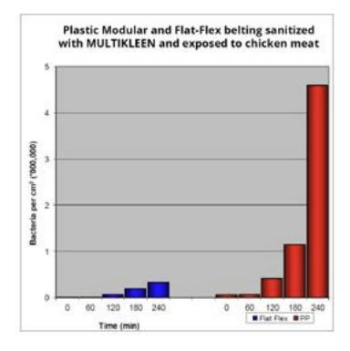
Research in the UK shows that with fish and meat Flat-Flex picks up fewer bacteria, maintains a lower level of contamination over time and is easier to sanitise, possibly because the gaps in plastic modular belting cannot be as readily cleaned as the stainless steel belting and harbour bacteria with quicker recontamination of the belt as a consequence. Drive shafts and the undersides of plastic modular belting are particularly difficult to clean in comparison with Flat-Flex belting.
